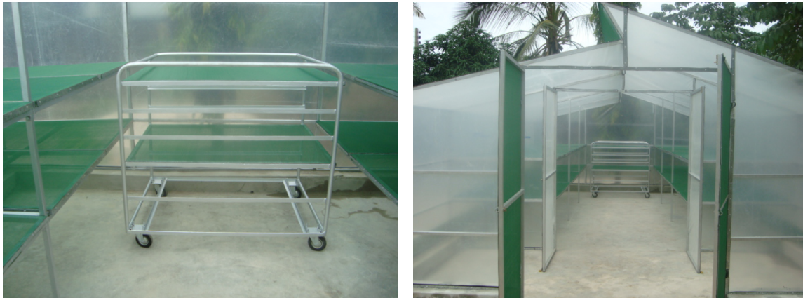
Figure 3: Trolleys inside the dryer utilized for transport of the products
