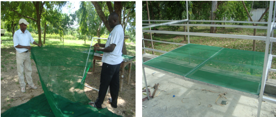
Figure 2: Fabrication of trays including cutting of plastic green wire mesh
