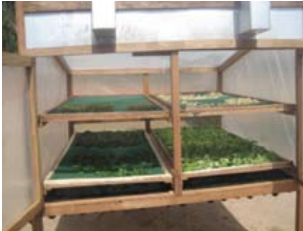
Drying vegetables using solar dryers
