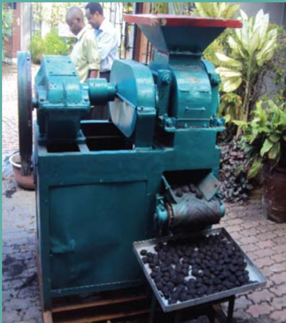
Briquettes produced from carbonized saw-dust and rice husk TaTEDO- Centre for Sustainable Energy Technologies and Services
